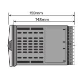
3508 Panel cut-out 92mm (-0.0 +0.8) x 45mm (-0.0 +0.6) 3504 Panel cut-out 92mm (-0.0 +0.8) x 92mm (-0.0 +0.8) Recipes
